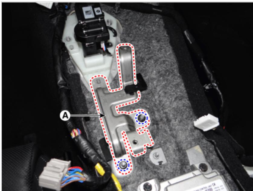
7. Disconnect the parking release actuator connector (A). Then, remove the cable by pulling it toward the vehicle interior.
